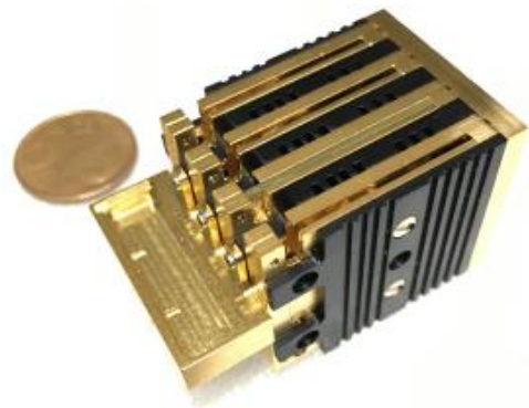
Assembly of 4 blades, including 16 RF channels, with part of the beamforming network.
